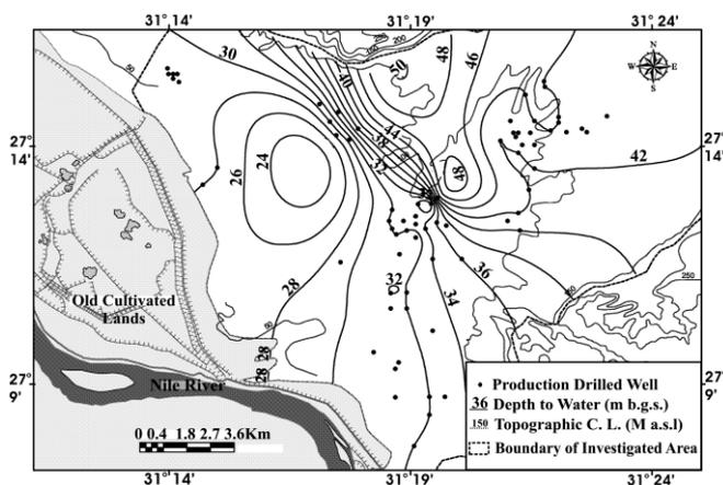
Fig. (5) Depth to water contour map of the Early Pleistocene aquifer system
