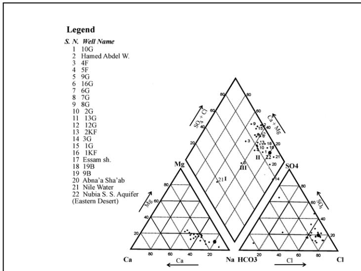
**Fig. (10) Groundwater hydrochemical evolution trend by Piper's trilinear diagram**
