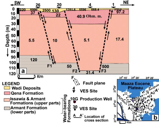
**Fig. (4) Illustrative subsurface aquifer situation by a) hydrogeophysical cross-section A-A' across Wadi El-Assiuti. b) key map of cross-section**
