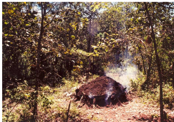
Figure 4. An oven for charcoal production.
