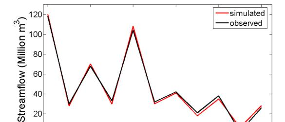
**Figure 3.** Observed and WEAP simulated streamflow time series at Rheraya catchment.
