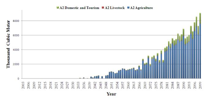
Figure 13 and Figure 14 show that, using the combination of the two proposed adaptation strategies, the water demand for domestic use, tourism and livestock sectors are fully met until2033 for A2 scenario and until2053 for B2 scenario. Supply for agriculture will fall short of demand for A2 and B2 scenarios. There are two reasons for the increase in unmet demand in the last decade of the study period. The first one is the increased demand due to higher per capita use rates and population growth,
