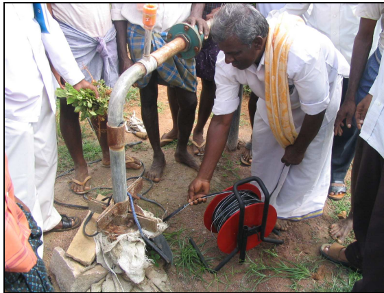
Fig.5: Participatory monitoring of groundwater levels
