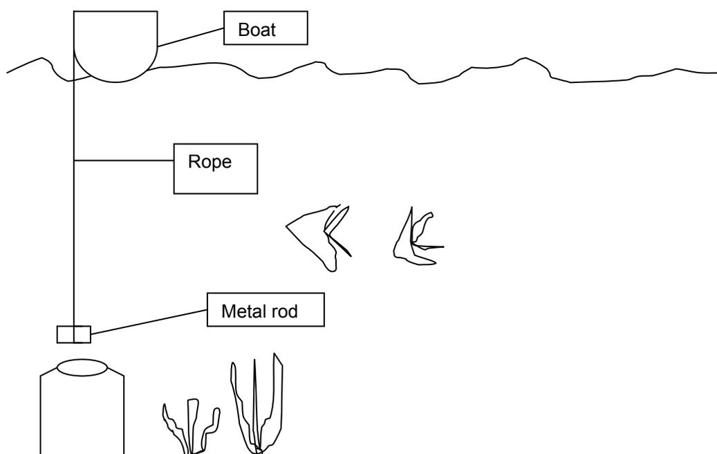
**Figure 3: Handling technique of the artificial reef**
