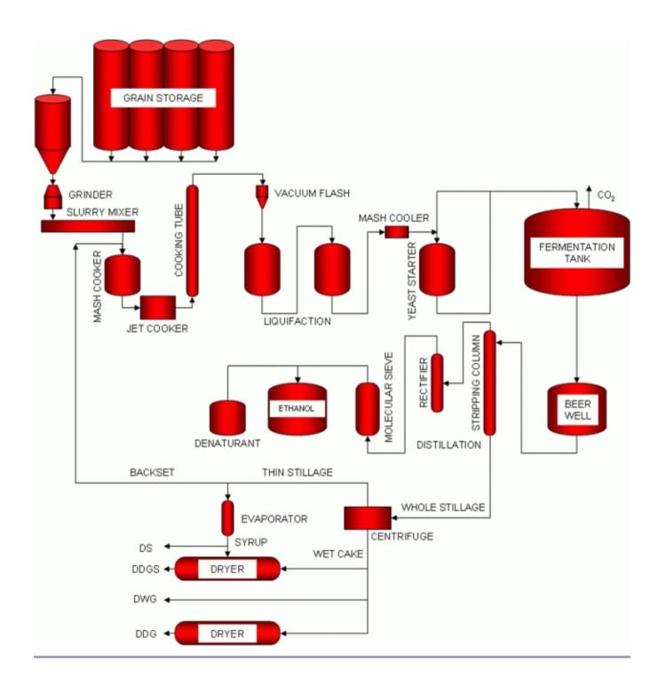
Fig. 3. Process flow diagram of corn-to-bioethanol manufacturing process.
