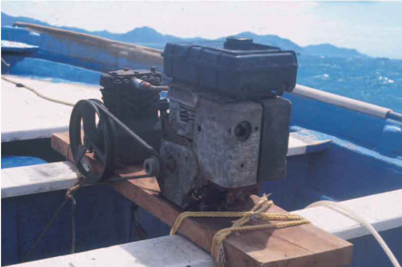
Figure 3. Hookah air compressor used by Canal del Infiernillo divers. (Photo by author)
