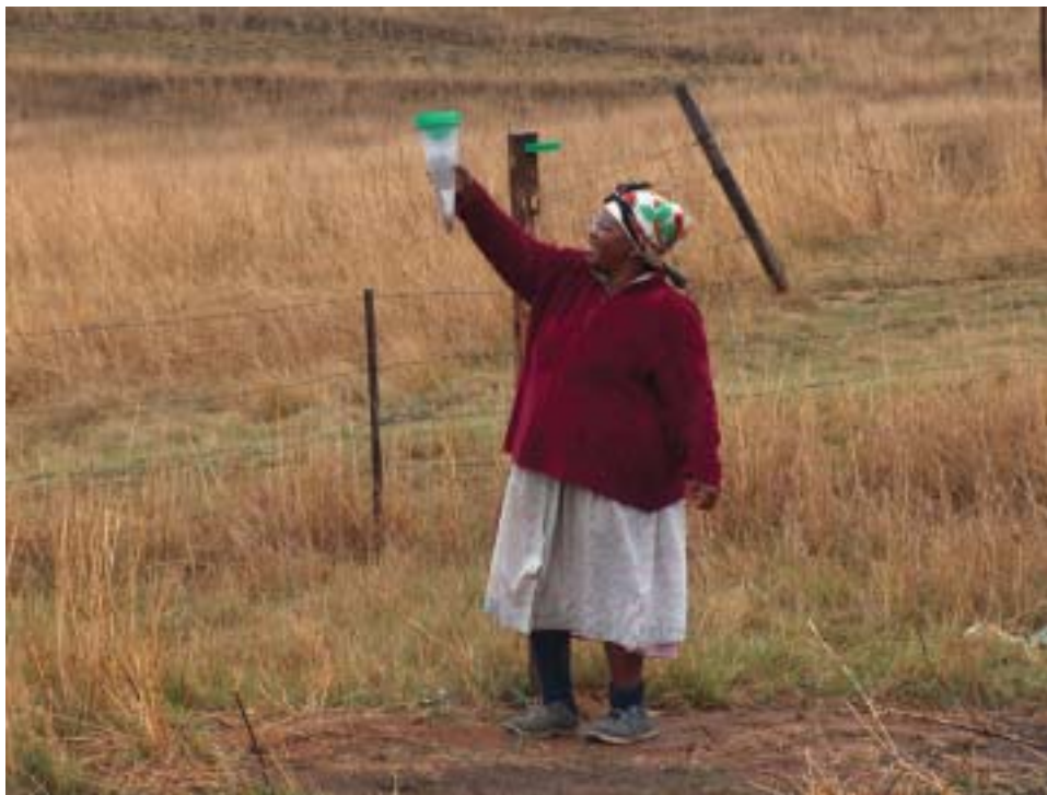
Figure 9. A smallholder farmer taking a reading from a manual rain gauge in Potshini.
