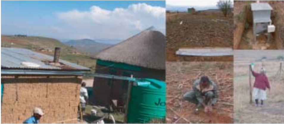
Rooftop run-off harvesting, setting up run-off plots, TDR access tubes and rain gauges.
