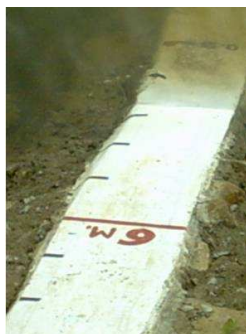
Figure 4: Calibrated gauge on the upstream side of the reservoir used to determine the stage of reservoir.
