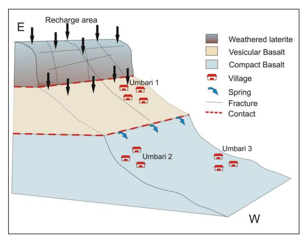
Figure 4: Conceptual layout of Umbari springs
