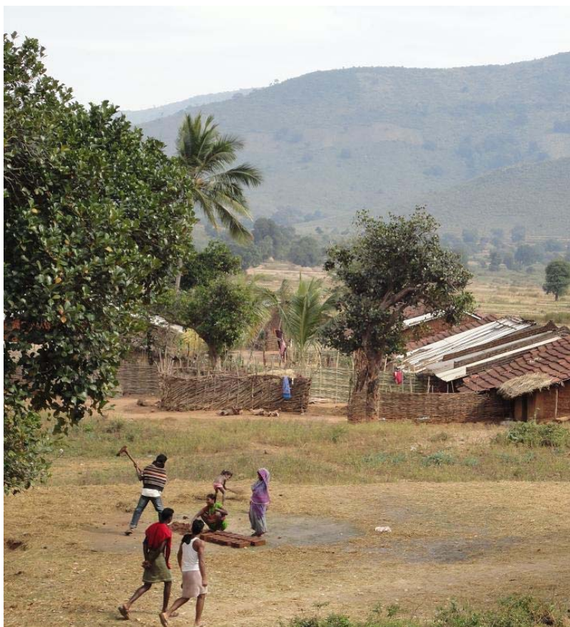
Baraja village, Orissa (India) : All the material for building the homes in this photo comes from the surrounding forest and land. Material for thatching the roofs and making the fences comes from the forest. The walls are made of handmade mud bricks and the photo shows women making these bricks.
