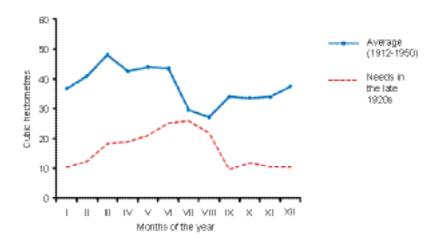
*Figure 1: Water available and water needed on the huerta of Valencia. Sources: http://hercules.cedex.es/anuarioaforos/afo/estaf-datos.asp?indroea=8022 (used to know the flow rate of the Turia) and Bellver (1933, 26–28).*
