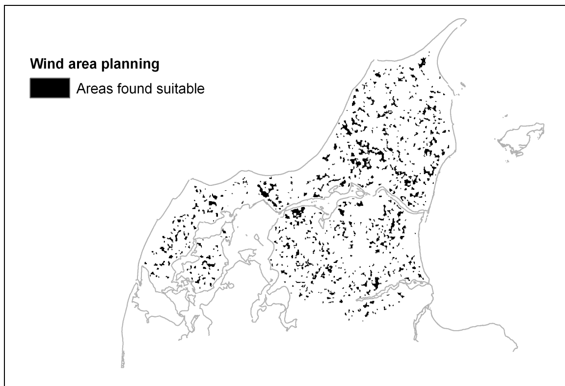
Figure 9: Areas which were found theoretically suitable for wind energy development, found by subtracting various exemption zones and buffers from agricultural land. The remaining area is 703 km 2 , equal to 8.9% of the land area.
