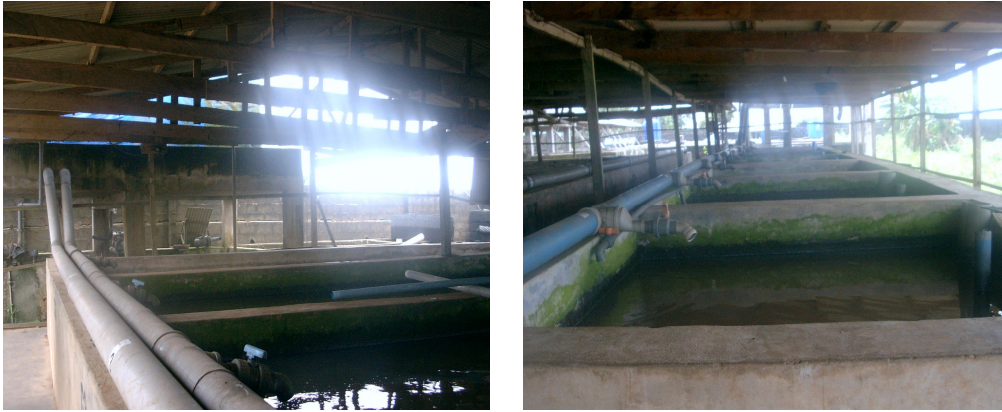
Fig. 5a & 5b. Interior of WRS facility for growing the African catfish, C. gariepinus in concrete tanks.
